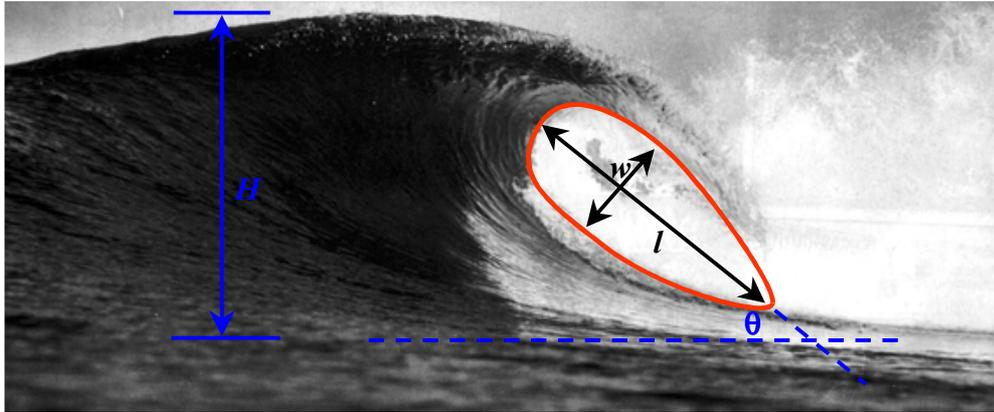
**Figure 6.1.** Curve fitting is applied to the forward face of a crest parallel wave image and used to calculate the vortex length ( $l$ ), width ( $w$ ) and angle ( $\theta$ ).  $H$  is the estimated wave height (after BLACK *et al.*, 1997).
