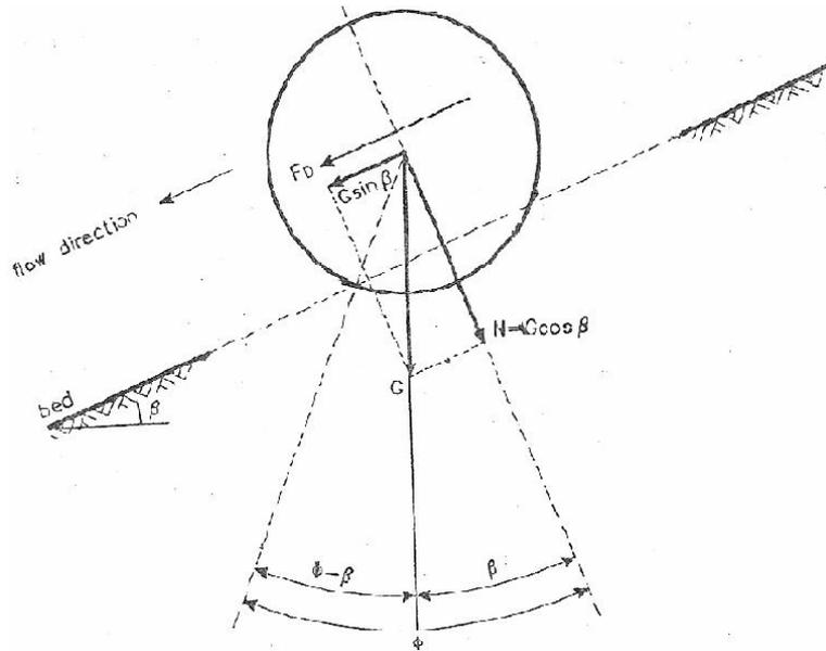
*Forces on a block (longitudinal bed slope) according to Von Rijn*
