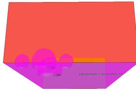
Boundary Conditions with StarCCM+: red= inlet, orange= outlet, purple = wall
