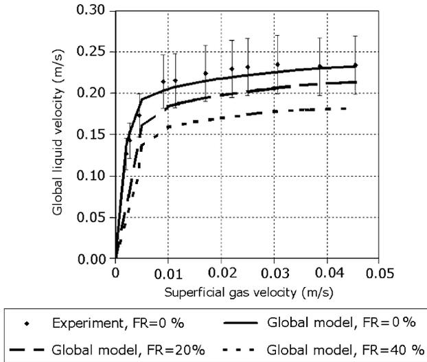
Fig. 8. Global liquid velocity.
