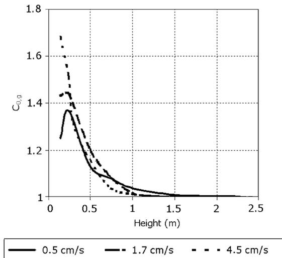
Fig. 3. Drift-flux coefficient in the riser.
