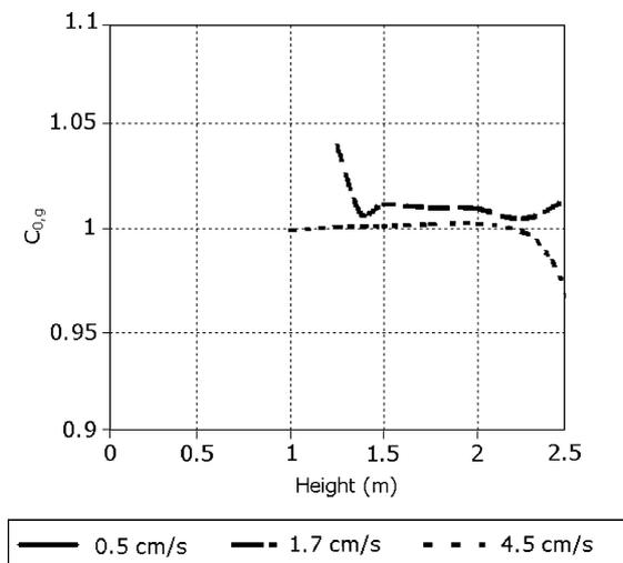
Fig. 4. Drift-flux coefficient in the downcomer.
